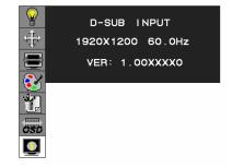
**Option 1:** OSD lock – All buttons except the Power button are locked. Press Exit key + Menu key + Soft power key at same time.
